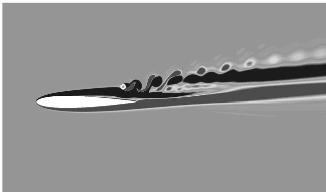
Fig. 11 Vorticity field around the NACA0012 airfoil and cylinder regions.
